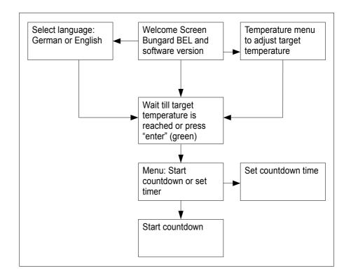
After switching on the mains the welcome screen "Bungard BEL" appears on the LCD and the software version
