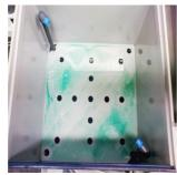
6. Now you have access to e.g. the etching nozzles adjustment
