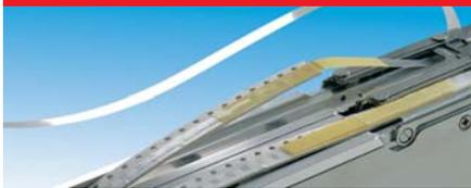
Every SMD tape needs a length of cover tape 'tail' for getting started in a feeder. When a partially used reel is to be used that does not have a leader tape, creating a 'tail' has up to now caused some components to be lost while peeling off the cover tape. To avoid this wastage, the cover tape is extended by applying a Steierform Cover Tape Extender! Steierform Cover Tape Extenders are available ex stock in the sizes 5 x 396 mm, 9 x 396 mm, 18 x 396 mm and 34 x 396 mm.
