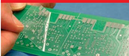
When printing or dispensing solder paste or adhesive in the set up phase machine parameters can be checked by printing/dispensing not on the PCB direct but onto a highly transparent, single sided adhesive foil Steierform 87-50201, temporarily attached to the board. This avoids having to clean PCBs - the foil can be easily removed without leaving any adhesive residues. Available in different sizes.
