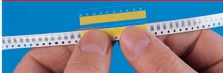
8 mm paper tapes are conveniently joined using Steierform SMD Double Splice Tapes. No fixtures or tooling are required as alignment of the component tapes to be joined is taken care of by the integrated positioning aid. This patented product, developed together with Siemens AG, joins the cover tape from the top as well as from below the component tape at the precisely maintained original pitch spacing! Available ex stock in size 22 x 40 mm (500 pieces/carton).
