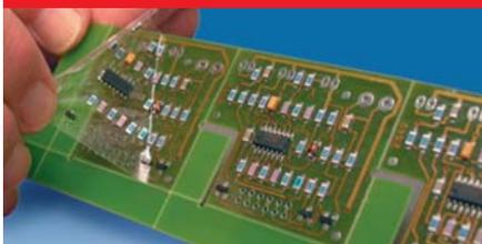
When setting up a pick and place machine the first off run is often carried out by placing SMDs onto a thin, highly transparent double sided adhesive foil Steierform 87-92403. The position, orientation and presents/absence of components can then be manually or automatically inspected. The foil is removed without adhesive residues being left on the surface of the PCB. Expensive component can be reclaimed for further use. Available in different sizes.
