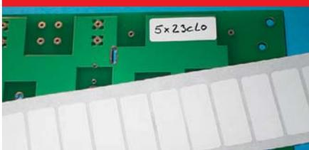
For the unambiguous identification of printed circuit boards thermally resistant Labels, Steierform 87-82003 (total thickness 0.045 mm) or Steierform 87-82004 (total thickness 0.08 mm) can be used. The polyimide foil, coated white, can be durably printed with thermal transfer printers and suitable thermal transfer ribbons.
