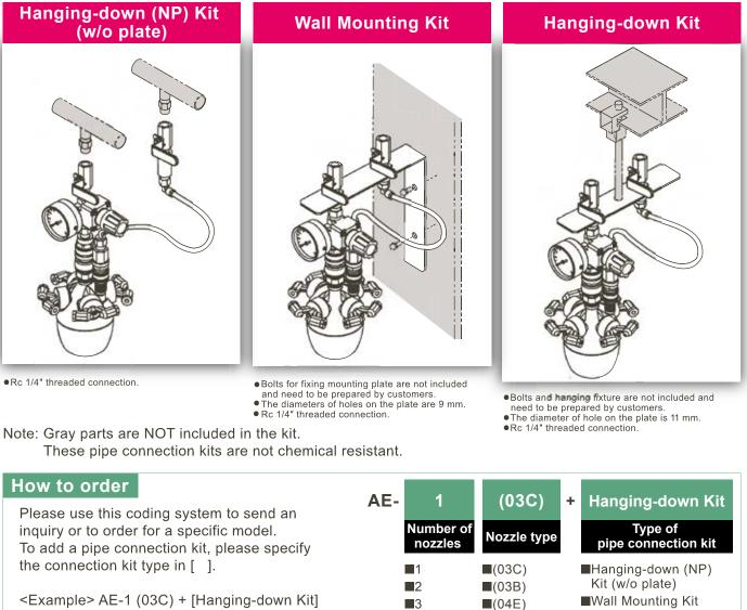
Note: Up to four nozzles can be mounted on one AKIMist® "E".
