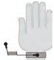
Anschlüsse für Armband / connection for wrist strap
