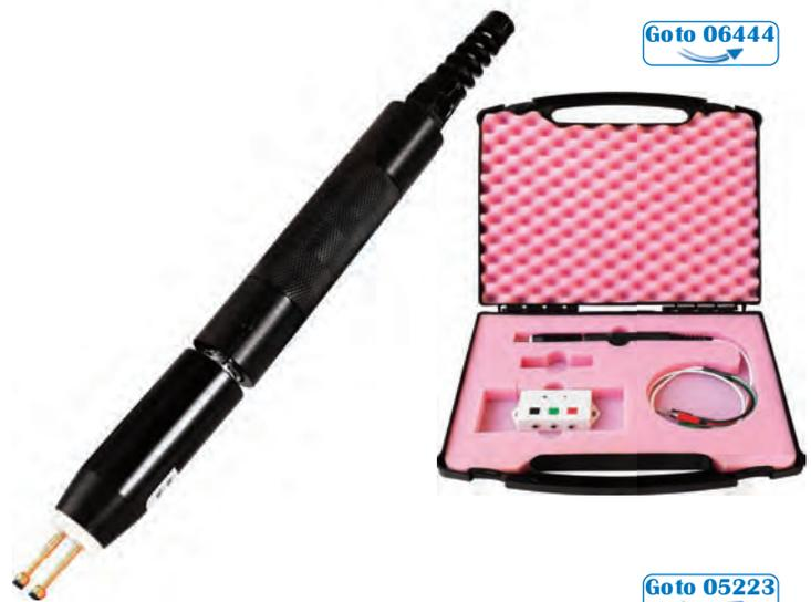
Adapter zur Verbindung von Zweipunktelektrode und Safe-STAT® RM 200, Safe-STAT® RM 1000, Safe-STAT® RM 4000 und Safe-STAT® Resistivity Meter, / connection adapter for two point electrode with Safe-STAT® RM 200, Safe-STAT® RM 1000, Safe-STAT® RM 4000 and Safe-STAT® Resistivity Meter
