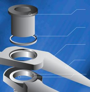
Nut is very strong, tough and hardened to resist high cutting loads
