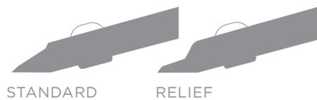
Cutters with relieved (low profile) heads permit increased access to confined areas. See photos for the difference between a standard cutter and a cutter with a relieved head.
