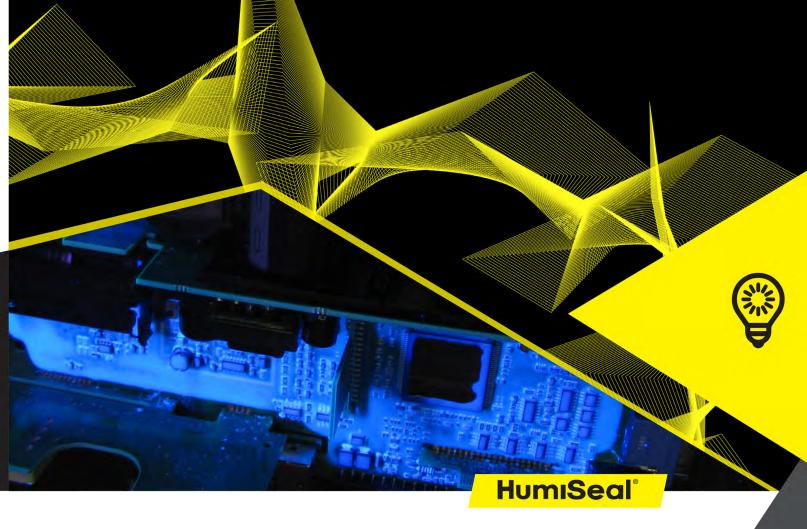
The latest LED curable UV coatings. UV300A series coatings are one-part, high solids, dual-cure acrylated polyurethane conformal coatings, possessing all the performance benefits of the original Humiseal UV coatings, but with the additional benefit of LED cure capability.
