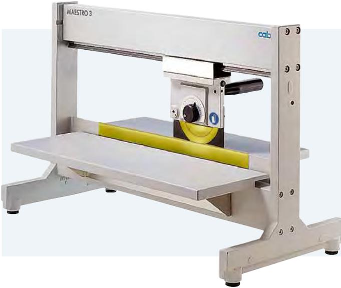
The MAESTRO 3E separates both small and large PCBs. The support table and the rest can be set continuously to the best possible operational position. By adjusting the distance between the linear blade and the rest, margin strips can fall through and are sorted out.
