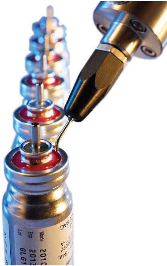
TS5440 - Dispensing medical device adhesive
