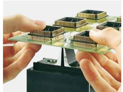
Hektor separates milled PCBs carefully and fast. The off-cut material is removed smoothly and precisely. The matrix consists of two parts. This ensures easy and cost-saving change of the blades. Compressed air is used for the separation process. The operating pressure can be set on the machine. When the foot switch is pressed, the off-cut is punched out. The off-cuts are collected in the collecting box. When the gate is opened the waste material can be extracted.
