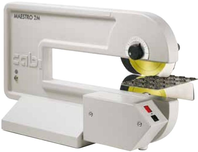
MAESTRO 2 separates small amount and prototype series of PCBs fast and economically. The compact and stable aluminum frame requires only a minimum of space.
