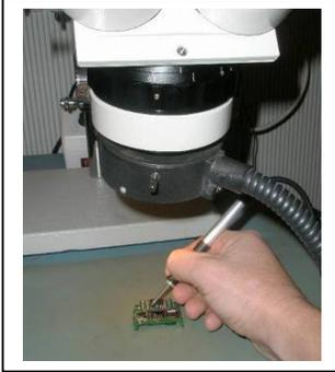
The size of the UFTC cartridge makes it easy to use in very restricted areas and under microscopes.
