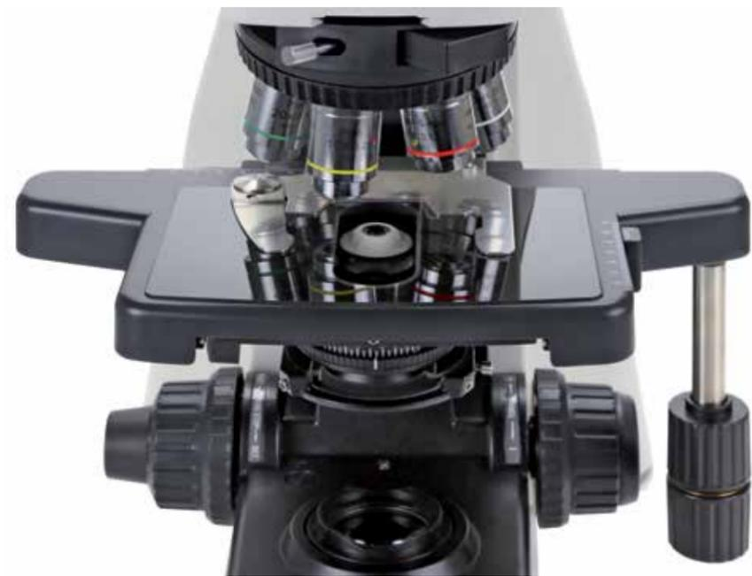
*Optional: mechanical stage with scratch-resistant Sapphire glass*
