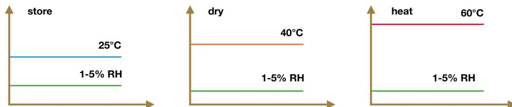
Stopping the moisture absorption and maintaining the remaining processing time.
