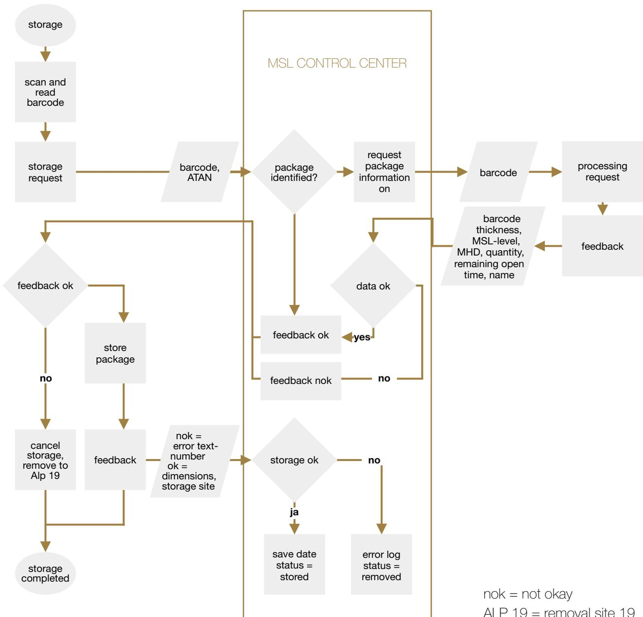
\*Sample layout of interface communication between Dry Tower and MES system (storing process).
