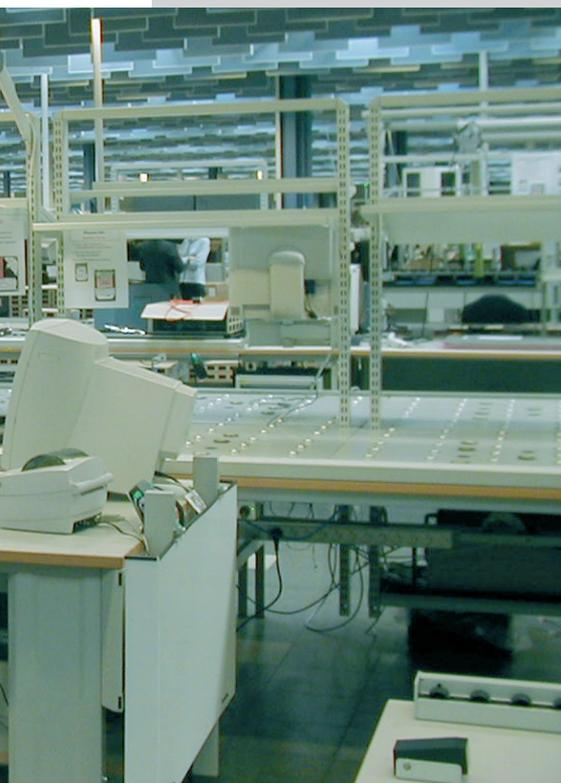
The **electronics assembly** industry is characterized by a large number of small, light components, requiring accurate, precise handling, precisely planned processes and tasks, and a short product lifecycle. Therefore workstations must be well organized and ergonomic. Product testing is often integrated with an electronics assembly line, so the transfer lines must meet ESD standards. The electronic products have a short lifecycle so production investments must also have a short payback time.
