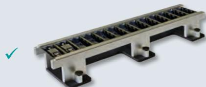
✓ All these feeders can be placed in the assembling area by magnetic bases.
