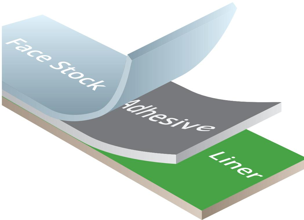
**Face Stock:** 2.3 mil gloss white polyimide with ultra durable chemical and high temperature resistance. The material is specifically designed to withstand multiple harsh chemical wash cycles in printed circuit board (PCB) manufacturing and also perform without preliminary heat treatment.
