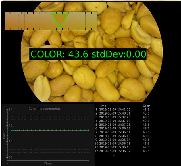
The average color value of the sample is written on the screen and displayed on the defined color range (top left corner) in green if within the defined pass limits. Standard deviation is also counted.
