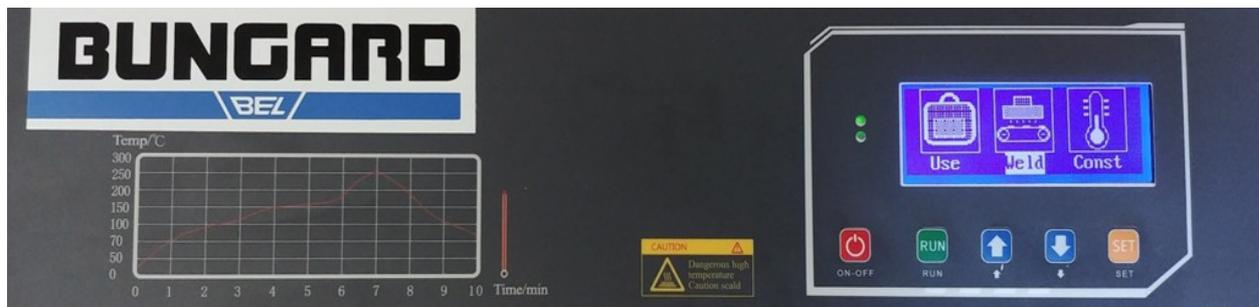
There are 5 buttons on the front panel of the unit: **POWER**, **UP**, **DOWN**, **SET**, and **RUN**, with the **RUN** and **SET** buttons being multifunction buttons. Depending on the dialog, there are various commands above the keys that are activated by pressing the keys.
