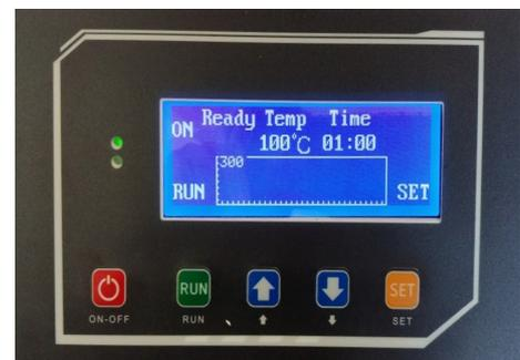
For **HOLD**, the holding time, the same applies, but the temperatures can only be adjusted between **100** and **220 ° C** here.
