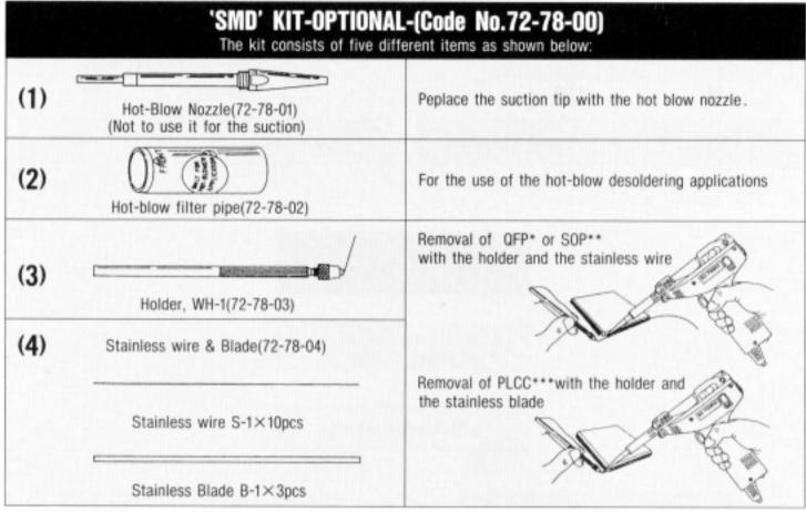
\*QFP:Quad Flat Package \*\*SQP:Small Out-line Package \*\*\*PLCC:Plastic Leaded Chip Carrier
