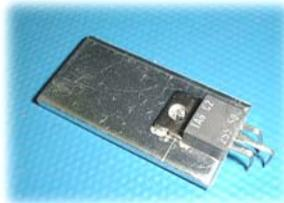
gas bubbles of the liquid solder and produces a shrinkhole free joint. This is very interesting for applications in high-vacuum.
