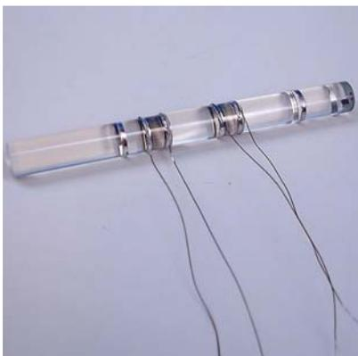
Contacting of Niob coil to a Zerodur rod
