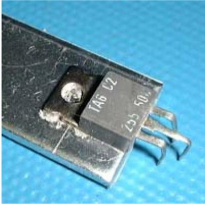
Soldering of power semiconductors on a cooling element (aluminum, aluminum oxide, ceramic etc) to provide best possible thermal connection.
