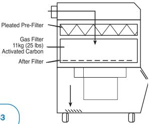
The MFX-2200G Fume Extraction System has been specifically designed for the removal of gases and vapors from a range of heavy duty bench-top applications, including solvent cleaning, gluing/bonding and conformal coatings.
