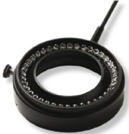
Ring-light containing 40 white LEDs for bright and homogenous illumination of objects. Designed for assembly on Optilia W10x and W10x-HD cameras. The compact control unit features an ON-OFF switch, brightness control and two outputs for connection to LED illumination units.
