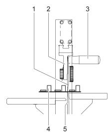
Fig. 10 Separating the PCB's
