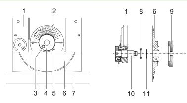
Fig. 11 Replacement of the upper blade
