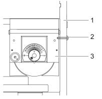
Fig. 4 Releasing the Upper Blade Lock
