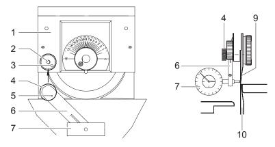
Fig. 7 Check the blade alignment
