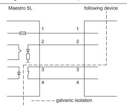
Fig.27 Interface to the following device
