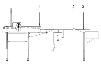
Fig.15 Operation with external Conveyer Belt
