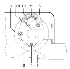
Fig.22 Blade Adjustment
