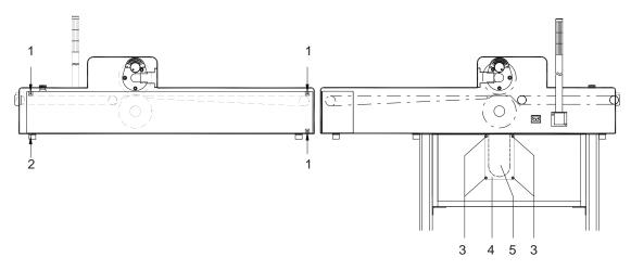
Fig.19 Replacement of the Lower Blades
