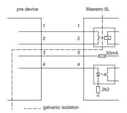
Fig.26 Interface to the pre device
