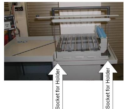
On the surrounding frame the Splash-Center has two small pieces of dark grey PVC in front of the tanks. These provide a stand for the board holder, so you have both hands free for placing the PCBs in the holder.
