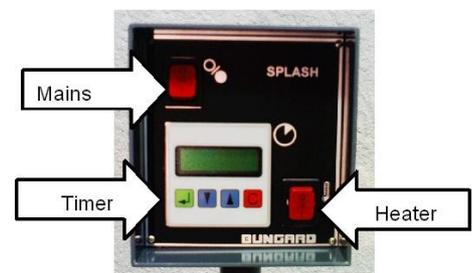
8. For a first test of the machine fill the spray chamber up to the sieve with water. Fill the rinse and treatment tank, each with about 10 liters of water.
