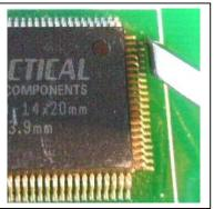
reworking with one of Metcal's hoof cartridges or any other type of equipment. Removal of these shorts is very simple following these steps.
