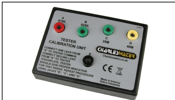
Figure 1. Charleswater 99090 Calibration Unit
