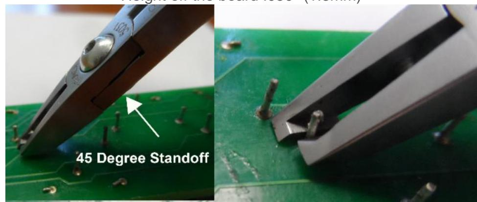
Tronex Model 5031 Standoff Cutter: 45 Degree Angle
