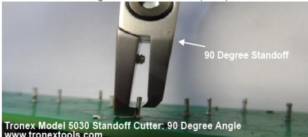
Tronex Model 5030 Standoff Cutter: 90 Degree Angle
