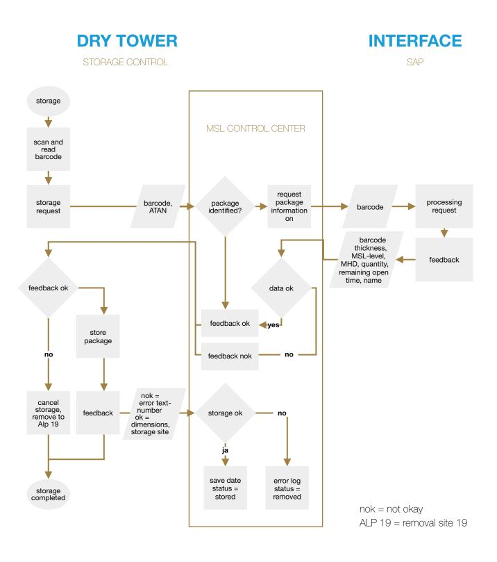
\*Sample layout of interface communication between Dry Tower and MES system (storing process).
