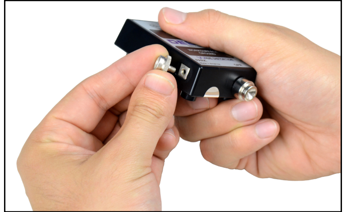
Figure 6. Changing the park snap on the 19243 Mini Monitor
