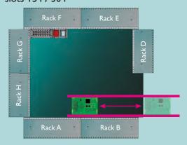
**SMD** fully automatic Pick & Place system with one Pick & Place head with lasercentering for 0201 chips up to  $22 \times 22$  mm (alt. up to  $32 \times 32$  mm) pitch 0,6 mm
