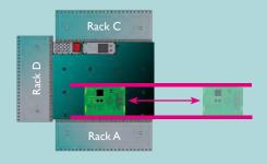
**SMD** fully automatic Pick & Place system with one Pick & Place head with lasercentering for 0201 chips up to  $32 \times 32$  mm, pitch 0,6 mm
