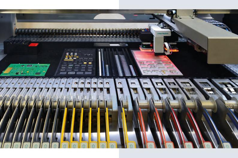
The placeALL®620L has a wider placement space than the placeALL®620. As a result, up to 284 feed positions and a maximum of 6 trays can be made available for production. The entire assembly room can also be used to assemble several small or large circuit boards (up to 910 x 430 mm).
