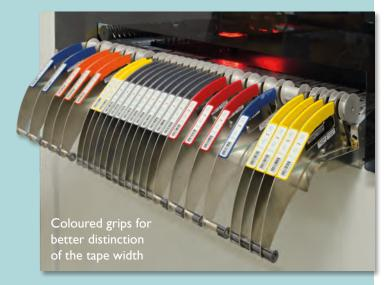
The placeALL® range of fully automatic machines offers the right feeder for every SMD model. The feeder system includes feeders for rolls, sticks, trays and for loose components and is available for all automatic machines.
