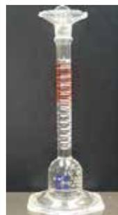
**STEP 5:** Immediately remove stopper. Wait five (5) to ten (10) minutes for the sample to separate (split) in the flask. Sample is complete when large bubbles completely rise to the surface.
