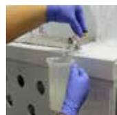
**STEP 3:** From the sample port, pull a 500mL sample to purge the sample line. Repeat if necessary to completely purge the sample line.
