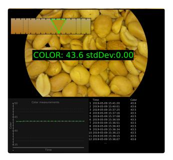
The average color value of the sample is written on the screen and displayed on the defined color range (top left corner) in green if within the defined pass limits. Standard deviation is also counted.
