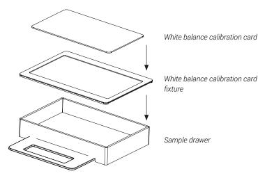
Then, insert the sample drawer with calibration card fixture and calibration card into the sample drawer positioner and press the white balance calibration button on the monitor to start the calibration.
