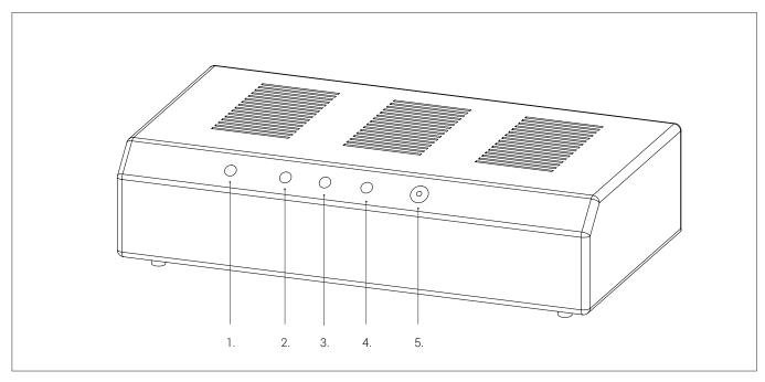
The controller connects the microscope to the XY table. By communicating with the controller, the microscope will systematically display all grids in the larval counting bassin.
