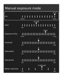
These settings will also be activated in Auto exposure mode. Otherwise, exposure compensation is the only setting visible. Iris, gain and exposure time will automatically be adjusted to recommended settings and cannot be adjusted in this mode.
