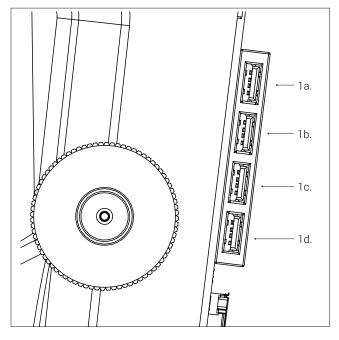
On the Trichinoscope is a USB Hub (1a-1d). Start by connecting this (2). Now, connect the mouse, USB key or USB hard drive to one of the other USB 2.0 ports in the USB Hub (1b).
