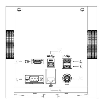
Connect the control box to the foot switch and then the foot switch to the Trichinoscope using D-SUB cables (4).
