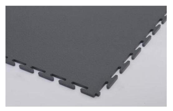
These interlocking floor tiles are made of PVC and during the molding process metal particles are injected. That way a very homogenic and durable conductive effect is generated, lasting the full lifetime of the product, considering wear and tear, unless correctly maintained by cleaning with antistatic floor cleaner.
