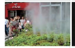
Energy-saving, outdoor cooling system with Semi-Dry Fog®, which provides effective evaporative cooling effect without wetting people.
