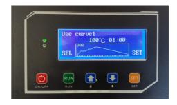
With **RUN** you leave the setting mode and with the arrow keys you switch back and forth between **READY**, **HEAT**, **WELD**, **HOLD** and **COOL** in the mode Soldering (**WELD**).
