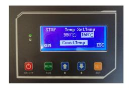
When the set temperature is reached, the indicator changes to green and the oven keeps the temperature.
