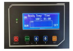
After **HEAT**, the soldering phase **WELD** starts, then the holding time **HOLD** and then automatically follows the cooling phase **COOL**. The fan turns on and a timer shows the elapsed cooling time.
