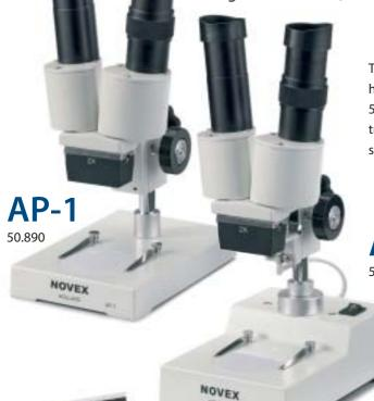
The AP-1 and AP-2 stereo microscopes have a vertical binocular head with dioptre adjustment and adjustable eye separation of 55 to 75 mm. Focussing movement is adjusted by two knobs via a transmission clutch. The stand is made of light metal and is supplied with black-white stage plate.
