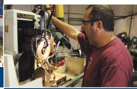
Surface grinding at Tronex insures exceptionally sharp cutting edges.
