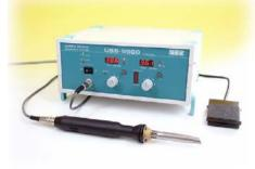
Ultrasonic-Frequency: Ultrasonic-Power: Temperature range: Heater: Heater power: Mains input power: Mains Voltage: Dimensions in mm - Base-Housing: - Hand tool: Soldering-Tip diameter: 40 kHz ±3 kHz 4 - 20 W ±2 W 150°C - 500°C Ceramic 100 W max. 200 W 100V - 260V / AC 48 - 65 Hz
