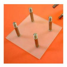
Mechanical joining of titanium rods on sapphire plate
