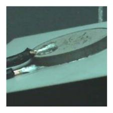
Applying of the metallisation Ø 20mm with solder in the centre of the aluminum-oxide plate. Producing at the same time a solder terminal/pad outside the piezodisk dimension.
