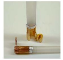
Hermetically sealed mechanical joining of gold plated component on a sapphire tube.
