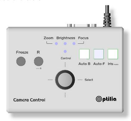
Joystick Left/Right: Switches between Zoom, Brightness and Focus functions.
