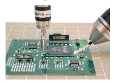
Flexia BGA Inspection System consist of Basic Flexia microscope unit, low aperture side viewing BGA zoom lens with built-in LED illumimation, external background illumination, extra SMT/PCB inspection 1-60x macro zoom lens and specially designed focusing stands.
