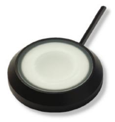
Backlight containing 20 white LEDs for bright, flicker-free and homogenous transmitted light or background illumination. The compact control unit features an ON-OFF switch, brightness control and two outputs for connection to other LED illumination units.
