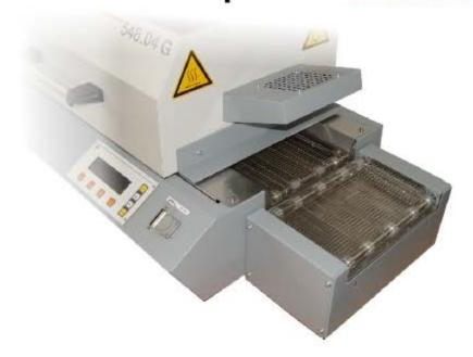
The transfer elongations allow an extension of the grid belt conveyor for approx. 20 cm and 30 cm respectively. Therewith a longer distance is available for the cooling of the PCB after the soldering process which is sometimes necessary when using lead free temperatures. The transfer speed is based on the adjusted speed of the soldering system because the TFV 200 will be connected parallel to the soldering system motor.
